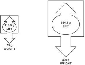
Smaller balloon lift from the heated air = 110.5 grams Lift available for payload = lift - envelope weight = 110.5 - 75 =
